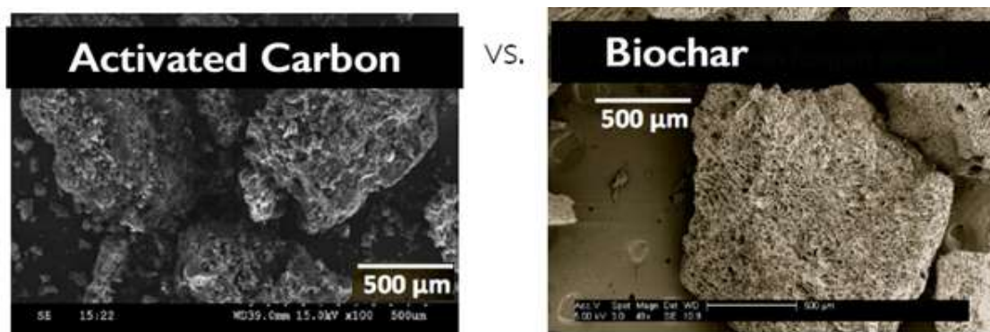
Figure 3: Activated carbon vs Biochar as adsorption media
